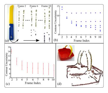
Figure 16: Disambiguation via accumulation. The toy knife is rotated by a robot arm with a known motion, 5 degrees in each frame. (a) The accumulation process of a knife. (b) Uncertainties of contours during an 8 frames of accumulation. (c) Mean and standard variation of uncertainties of contours in each frame. (d) An accumulated toy basket.
