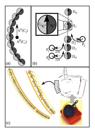
Figure 5: Illustration of contour attributes. (a) Orientation and position of a sample contour. (b) Calculation of mean color for a contour. (c) Mean left and mean right colors of two 3D sample contours.
