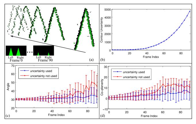
Figure 7: Effect of uncertainty on contour relations for the isosceles sides of the triangle in an artificial dataset. (a) Some samples from the dataset as stereo image pairs and 3D primitives. (b) Change in the contour uncertainty as the triangle moves away from the camera. (c) The angle between the sides of the triangle as it moves away from the camera. (d) The coplanarity between the sides of the triangle as it moves away from the camera.
