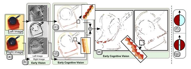
Figure 1: An overview of the hierarchical visual representation. (a) Stereo image pair, (b) Filter results, (c) 2D primitives, (d) 2D contours, (e) 3D primitives (shown in our 3D displaying software), (f) A 2D edge primitive, (g) A 2D line primitive.
