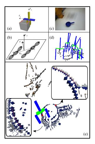
Figure 13: Grasping with a two-fingered gripper. (a) A grasp is defined by a location and two directions  $(r_1,r_2)$ . (b) The direction vectors for local features are defined as  $r_2 = (u_3 \times u_1) + (u_2 \times u_3)$  and  $r_1 = u_3 \times r_2$ . (c) A blue pan to be grasped. (d) A set of grasping hypotheses generated to grasp the blue pan. (e) An example grasp based on contours.
