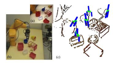
Figure 14: Grasping in a cluttered scene. (a) Objects to be grasped. (b) The robot grasps an object based on a grasping hypothesis. (c) A set of successful grasping hypotheses generated to grasp the objects in the scene.
