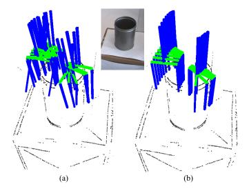
Figure 15: Grasp locations for different approaches. (a) Grasps that are calculated by using local features for different noise levels. (b) Grasps that are calculated by using contours for different noise levels.
