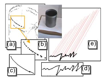
Figure 4: A sample 3D contour (a) 3D primitives. (b) 3D primitives of a selected part. (c) The 3D contour that contains the primitives in (b). (d) The contour in (c) from a different view point. (e) Dominant uncertainty directions.
