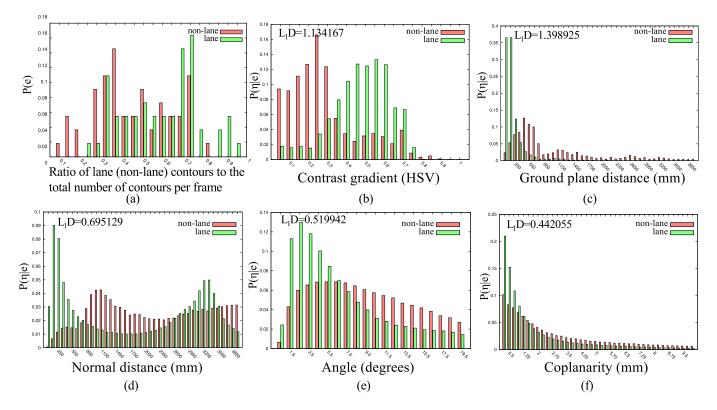
Figure 9: The prior probability distribution (a) and conditional probability densities (b-f) for relations between contours that contain a maximum of 6 primitives.
