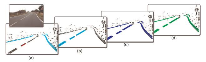
Figure 8: Illustration of 3D relational cues. (A selected 3D contour is marked in red in (a)). (a) All contours that have 1500-3500 mm normal distance to the selected contour. (b) All contours that have 0-200 mm normal distance to the selected contour. (c) All contours that are coplanar to the selected contour. (d) All contours that have  $0-5^{\circ}$  angle to the selected contour.
