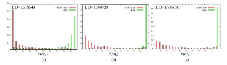
Figure 10: The normalized histograms of the posterior probability densities for individual and grouped entities. (a) Based on individual primitives. (b) Based on groups of maximum 6 primitives without uncertainties. (c) Based on groups of maximum 6 primitives after applying an uncertainty threshold.
