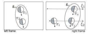
**Figure 8. The BSCE criterion.** Let  $\pi_1$  be a primitive in the left frame forming a group with a second primitive  $\pi_2$ .  $\pi_1$  has a stereo correspondence  $\pi_s$  that lie on the epipolar line  $\xi_1$  in the right image. Both  $\pi_i$  and  $\pi_j$  in the right image lie on the epipolar line  $\xi_2$  of  $\pi_2$ ; hence these two primitives are both putative correspondences of  $\pi_2$ . doi:10.1371/journal.pone.0010663.q008
