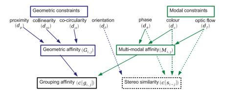
Figure 3. Illustration of the measures used in this paper and how they are combined. Solid arrows indicate the metrics used for stereopsis, dashed lines the metrics used for perceptual grouping. doi:10.1371/journal.pone.0010663.g003
