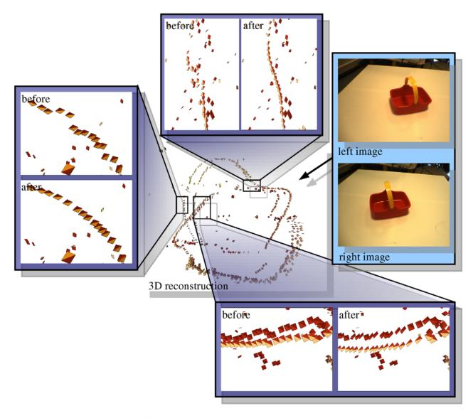
**Figure 19. Illustration of the effect of the correction of 3D primitives using interpolation.** The figure shows the reconstructed primitives before and after 10 rounds of correction, for details of an object. doi:10.1371/journal.pone.0010663.g019
