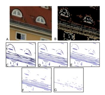
**Figure 5. Illustration of the links extracted for different affinity thresholds. A** detail of the original image ( $220 \times 280$  pixels); **B** extracted primitives; **C**–**G**. extracted links for values of  $\tau_A =$ (**C**) 0.1, (**D**) 0.3, (**E**) 0.5, (**F**) 0.7, and (**G**) 0.9 — using  $\mu = 5$ . The blue lines represent the links, where more saturated lines stand for higher affinity values.
