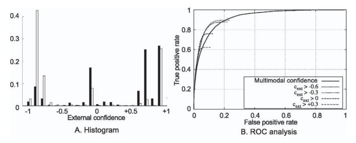
**Figure 13. Evaluation of the external confidence. A** Histogram of the external confidence rating for correct (black bars) and false (white bars) correspondences. **B** Each curve stands for a the application of a different threshold over the external confidence, prior to the ROC analysis. These curves represent the statistics over 10 frames of the three sequences with ground truth — see Figure 10 **A**, **B** and **C**. doi:10.1371/journal.pone.0010663.g013
