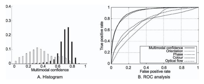
**Figure 12. Evaluation of the multi-modal stereo. A** Histogram of the multi-modal similarities between correct (black bars) and false (white bars) potential correspondences. **B** ROC curves for the different modalities. These results have been collected over 10 frames of the sequences Figure 10 **A**, **B** and **C**. doi:10.1371/journal.pone.0010663.q012
