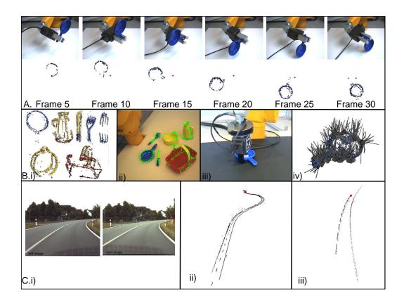
Figure 10: Applications. A) BoO: Show emerging object over different frames and the subtraction of gripper. B) Pose Estimation and Grasp Learning: i. Accumulated objects used for ii. pose estimation; iii. object grasping; and iv. storing of successful grasps. C) Driver assistance scenario: i. Stereo Image; ii. Outdoor map; and iii. accumulated lane.
