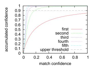
Figure 4: Confidence update for repeated observations of the same match quality. The x-axis shows the quality of the match and the y-axis the resulting updated confidence, for the five first updates. The dashed line shows the threshold we used for these experiments, i.e.  $\tau_{\text{max}} = 0.9$ . Above this value, the hypotheses were considered as confirmed.
