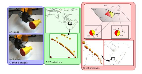
Figure 1: Illustration of the primitive extraction stage. A) original images (left and right); B) extraction of 2D-primitives; and C) stereo reconstruction of 3D-primitives.
