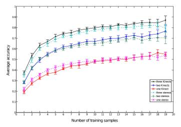
Fig. 6. Performance comparison of classification on single, double and triple views taken from both Kinect and Stereo cameras.
