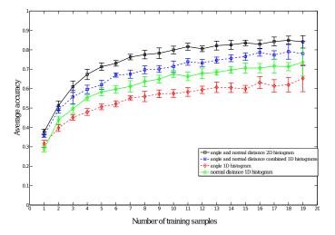
Fig. 8. 2D histogram of two features compared to combined 1D histograms, and when using only one feature at a time.
