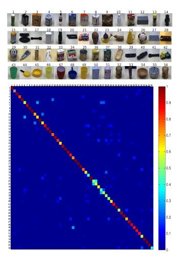
Fig. 5. Classification confusion matrix of 56 objects (shown above). It is obtained from a testing subset of 8 samples for each object while 12 samples are used for training. The visual representation is extracted from 3 Kinect cameras
