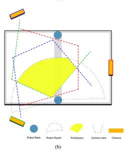
Fig. 1. The setup. (a) overview of the setup showing the robot arms and the camera pairs (the close-up view shows one pair of Kinect and stereo). (b) a top-view sketch for the setup depicting the workspace.
