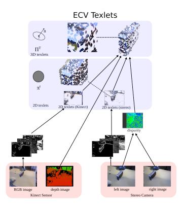
Fig. 2. The hierarchical representation of the ECV texlets. Example images from Kinect and stereo cameras are shown at the bottom. In the middle, 2D texlets are extracted after filtering operations. On top are the extracted 3D texlets from different cameras. This figure is best viewed in color.
