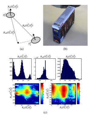
Fig. 3. Texlet relations. a) definition of shape relations between texlet  $\Pi_i^T$  and texlet  $\Pi_j^T$ ; Euclidean distance  $R_d(\Pi_i^T, \Pi_j^T)$ , angle  $R_a(\Pi_i^T, \Pi_j^T)$ , and normal distance  $R_{nd}(\Pi_i^T, \Pi_j^T)$ . c) relation histograms of all pairs of texlets extracted from object shown in (b).
