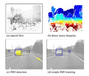
Figure 2: Illustration of the IMO detection level: a) the optical flow; b) the dense disparity; c) the low-level independent motion measure (yellow) and the detected IMOs after world-knowledge integration (blue boxes); d) the IMOs remaining after the simple tracking stage.
