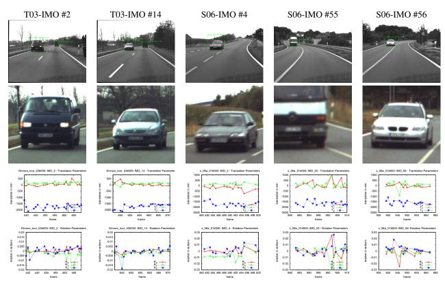
Figure 7: Example IMOs, two of which were taken from the sequence T03, and three from the sequence S06. The first row shows the detected IMOs; the second the high resolution ROI; the third the estimated translation, provided as  $T = (T_X, T_Y, T_Z)$ ; and the fourth the estimated rotation, provided as  $R = \alpha a$ , where  $\alpha$  is the rotation angle and a the axis.
