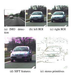
Figure 5: Illustration of the attention mechanism: In a) the detected IMOs are denoted by bounding boxes in the image (red for deleted spurious IMOs, green for valid ones). In b-c), the region of interest (ROI) extracted from the detected IMOs are shown. In d), the red arrows indicate extracted SIFT features. In e), the red lines indicate stereo-correspondences of 2D-primitives.
