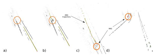
Figure 8: Illustration of a) the reconstructed road structure, b) and c) trajectories for the ego- and IMO-motion, and d) the reconstructed 3D model of the car with the lane structure.
