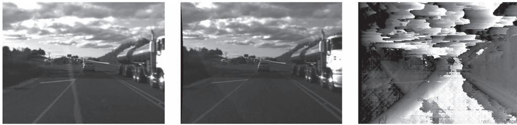
Fig. 2. Example of stereo input data (left and middle) and a disparity map obtained with SGM-BT (right). This disparity map is fairly useless in this particular case, and this condition illustrates a “bad performance.” Note that the cameras also record some reflections on the windscreen in this example of a situation that might be called “brightness differences between left and right images, and an approaching truck.” The first event (brightness differences) causes the BT cost function to fail, and the second event (approaching truck) should be solvable for the SGM matching strategy, in principle, when using a “better” cost function for matching than BT.
