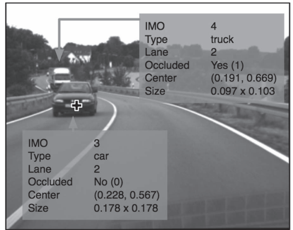
Fig. 10. Frame 875 of the Suburban Bridge sequence (left camera) shows two IMOs, for which hand-labeled data are provided. Furthermore, gaze positions are available, both in coordinates and classified targets. In the ego-vehicle, we observe the number plate of IMO 3 (black and white cross) and further data, also on IMO 4.
