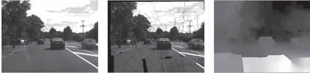
Fig. 4. Application for a sequence in set 5. (Left) Third view. (Middle) Virtual view for the disparity map shown on the right. The matching algorithm applied was BP stereo analysis. The specularities (left), which is apparent both in the recorded left and right images, causes a “defect” in the calculated disparity data.
