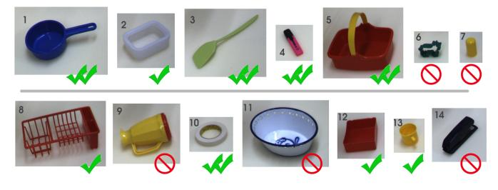
Fig. 12. Office and toy kitchen objects used in the experiments. Objects are of mostly uniform colours, and their size and the shape is suitable for grasping with the parallel jaw gripper. The marks illustrate average success rate in grasping individual objects measured in the experiments (see also table 3).
