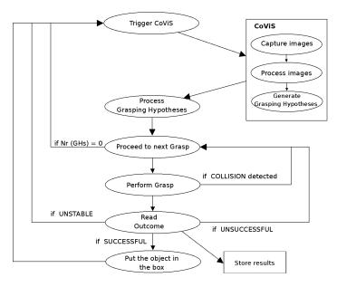
Fig. 10. State diagram showing work flow of exploration using the grasping behaviour.
