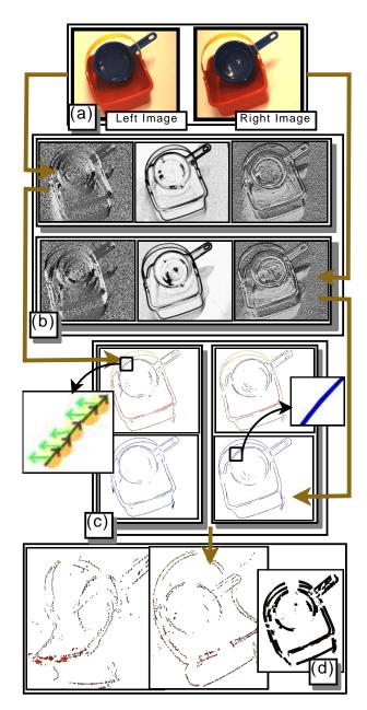
Fig. 2. Different type of information that is available in the representation. (a) Original stereo images. (b) Filter responses. (c) 2D primitives and contours. (d) 3D primitives from two different view points and 3D contours.
