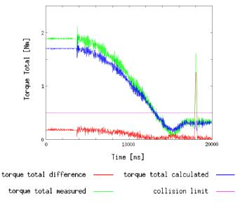
Fig. 9. The graph shows the total measured and the total calculated torques, and the difference between measured and calculated values as a function of time for a sample grasping attempt where a collision happened. Figure 13 shows an example collision situation and the corresponding grasping hypotheses.
