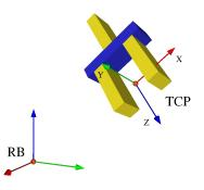
Fig. 7. The figure shows the Tool Centre Point (TCP) reference frame. It is given in respect to the robot's base (RB) frame. The position and orientation of the TCP reference frame is used when defining elementary grasping actions.
