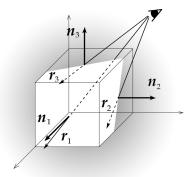
Fig. 6. Choosing the correct surface normal.  $\mathbf{n}_1$ ,  $\mathbf{n}_2$ , and  $\mathbf{n}_3$  are outward surface normals marking the sides of the cube visible on the illustration. The two sides visible from the marked point of view have surface normals  $\mathbf{n}_2$ , and  $\mathbf{n}_3$ .  $\mathbf{r}_1$ ,  $\mathbf{r}_2$  and  $\mathbf{r}_3$  are camera rays, vectors originating from the marked point of view and pointing to the surface normals.
