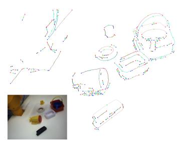
Fig. 4. 3D contours extracted from the scene that is shown in the bottom left (left image). Red dots indicate the first primitive in a contour, green the middle, and blue the last primitive in the contour.
