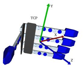
Fig. 17. A model of the five fingered anthropomorphic hand of the humanoid robot ARMAR-III. The shown TCP reference frame allows for a direct mapping to the EGAs produced for the two finger gripper (see figure 7). Please note that only one of the two possible orientations for a single EGA is shown (the not shown one is achieved by rotating the hand  $180^{\circ}$  around the z axis).
