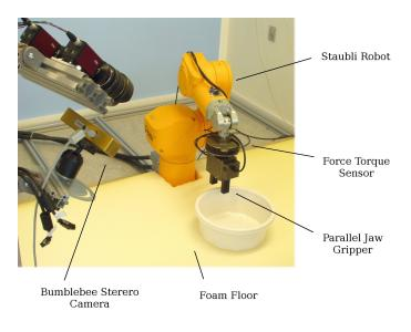
Fig. 8. Experimental setup.
