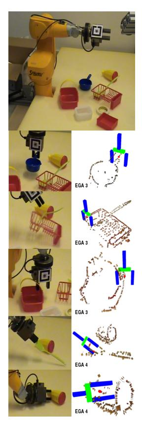
Fig. 13. Five grasping outcomes from the video available at [46]. From top to bottom: Successful, Unstable, Collision, Successful and Fail cases. A snapshot from the video (left) and the corresponding grasping hypotheses viewed in a visualisation environment (right) is shown for each case.
