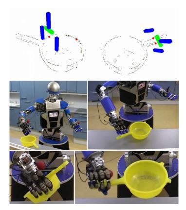
Fig. 18. Two executed grasps on ARMAR-III taken from the video [62]. From top to bottom: Predicted grasps, snapshots of the robot performing approaching movements, final configuration. Predicted grasps are shown from the point of view of the robot.
